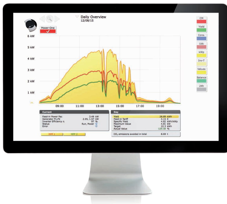
Keeping control - daily overview with two MPP-Tracker to ensure that the solar power plant runs efficiently.
